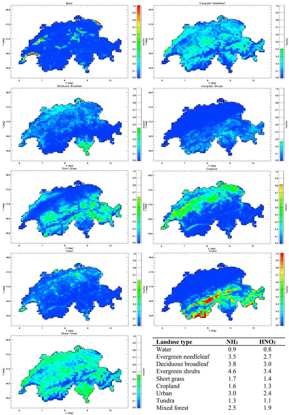
**Figure 5:** Fractional distribution of land-use types in grid cells of the Swiss domain and annual dry deposition velocities ( $\text{cm s}^{-1}$ ) of  $\text{NH}_3$  and  $\text{HNO}_3$  on these land-use types (Table).
