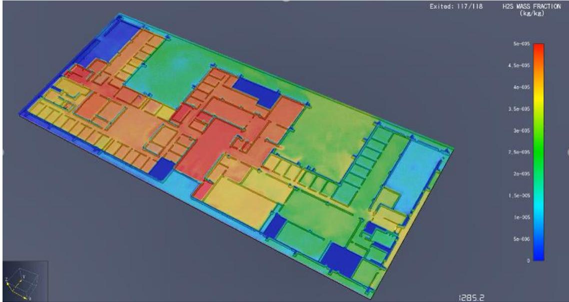
**Figure 1:** LES modelling of indoor dispersion of H<sub>2</sub>S in the administration building.
