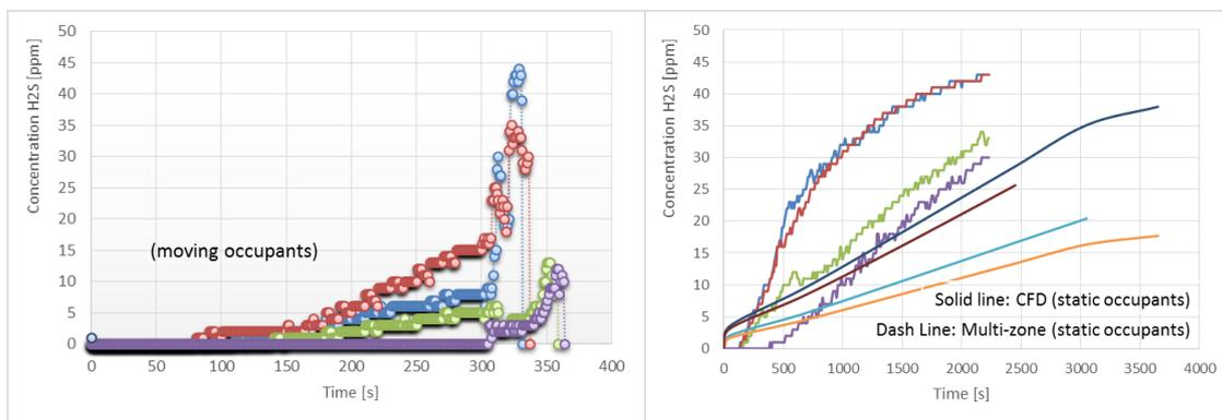
**Figure 3.** Toxic load estimation of the moving evacuees after a delay of 300 s: a) CFD results for moving occupants and b) CFD vs multi-zone (CONTAM) results for static occupants.
