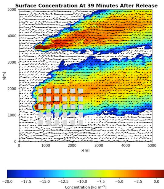
Figure 3. A side-by-side illustration of the surface concentrations and wind vectors for an open terrain area and within an array of thirty 20 m tall square surface obstacles.
