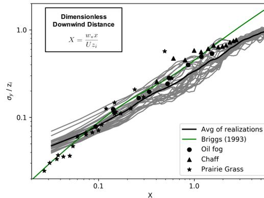
Figure 2. Plume crosswind dispersion vs. downwind distance.
