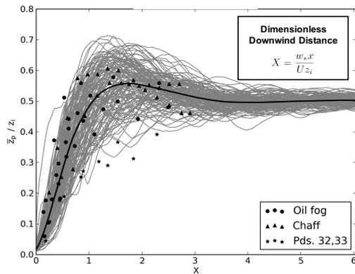
Figure 1. Plume height vs. downwind distance from the source.
