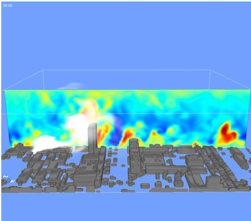
Figure 4. An illustration of a JOULES simulation of winds and dispersion over the TU Delft campus. The vertical cross-section illustrates vertical velocity.
