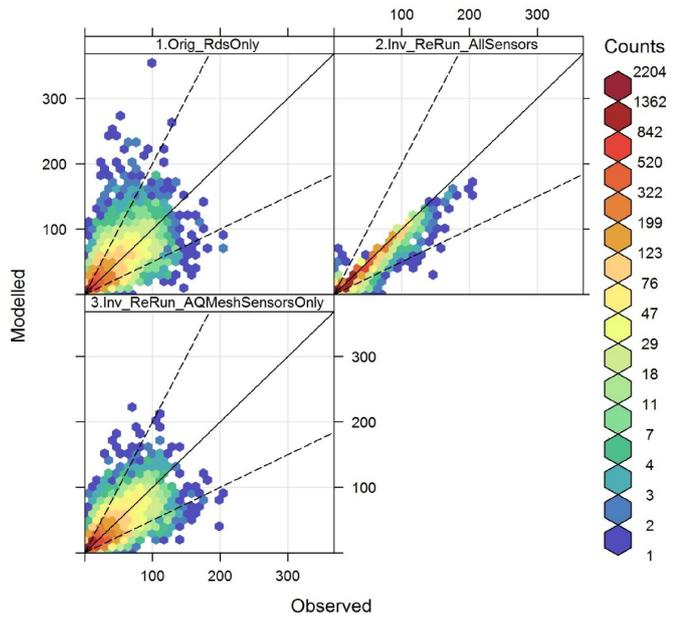
**Figure 3.** Frequency scatter plots of modelled versus observed hourly  $\text{NO}_x$  concentrations (ppb) at the reference monitors for three emissions cases: original emissions; adjusted emissions using all reference monitor and AQMesh sensor data; and adjusted emissions using AQMesh sensor data only
