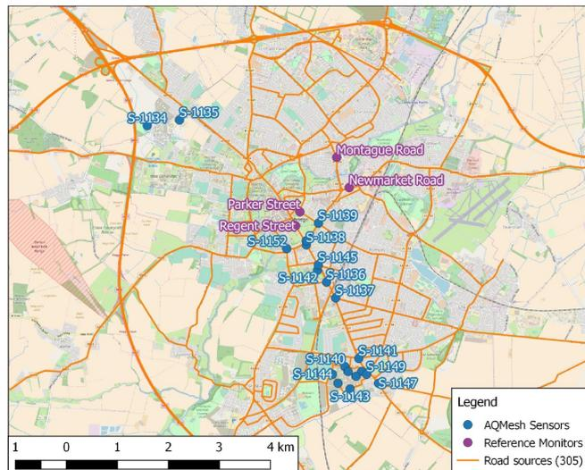
**Figure 1.** Map of Cambridge showing the locations of the AQMesh sensors, the reference monitors and the 305 road sources modelled.
