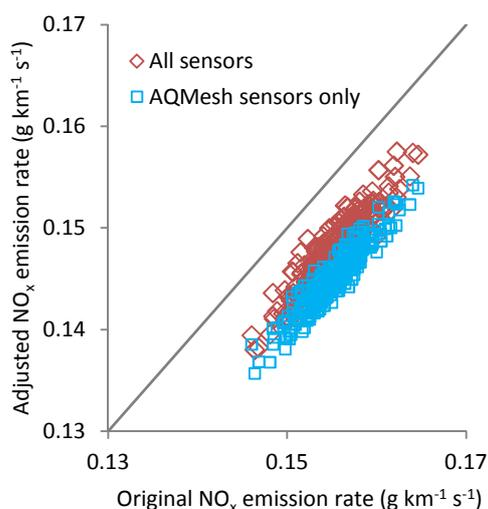
**Figure 5.** Scatter plot of adjusted versus original  $\text{NO}_x$  emission rates. The  $y=x$  line is shown in grey.
