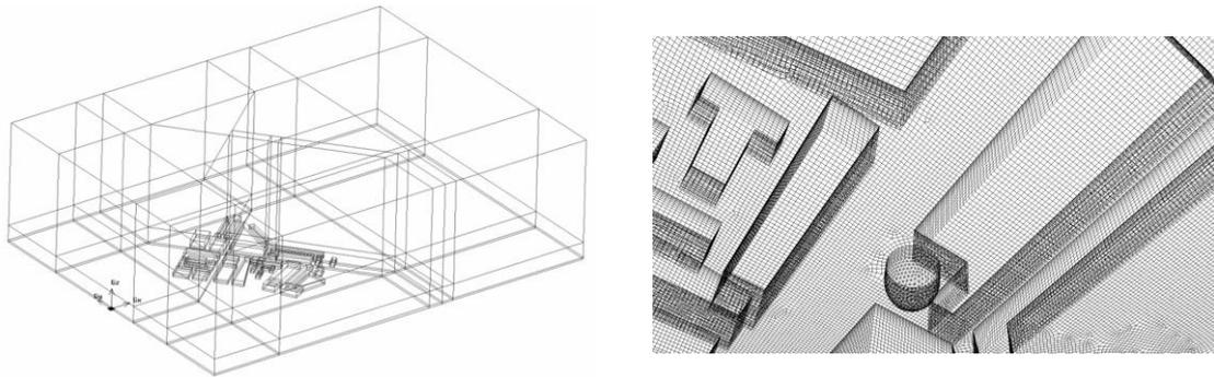
**Figure 3.** Computational domain (left) and some details of the structured mesh (right).
