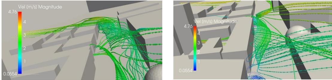
**Figure 4.** Instantaneous streamlines of the velocity field at the intersection (left) and in the middle of the canyon (right).
