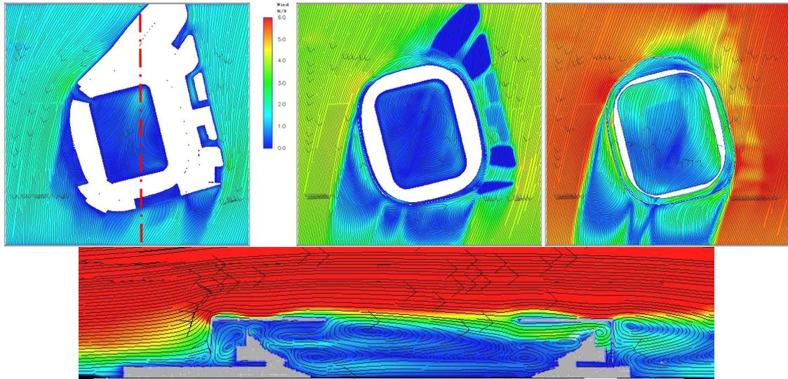
**Figure 4.** Horizontal and vertical cuts of the wind field on domain N03. The horizontal cuts are represented at a height of 4 m (middle of the lower rostrum), 13 m (middle of the intermediate stand) and 21 m (middle of the upper stand). The vertical section plane is indicated by the red line on the first illustration.
