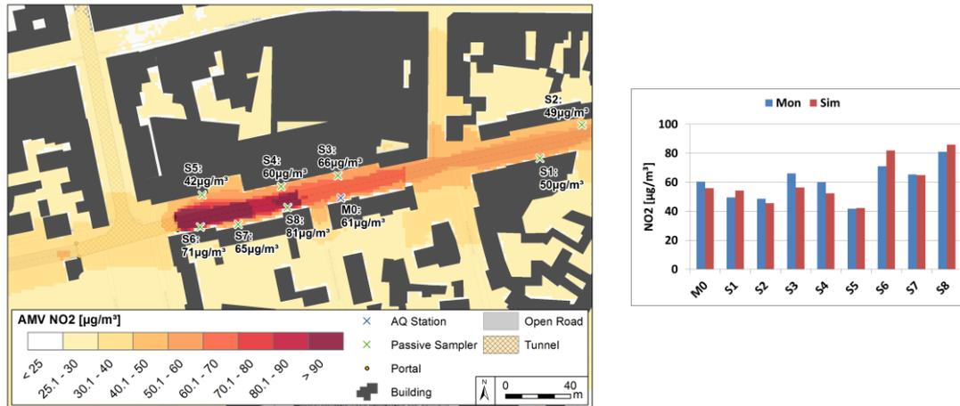
Figure 4. Simulated  $AM\ NO_2$  concentration and location and results of air quality monitoring (left) and comparison of monitored versus simulated  $AM\ NO_2$  (right).
