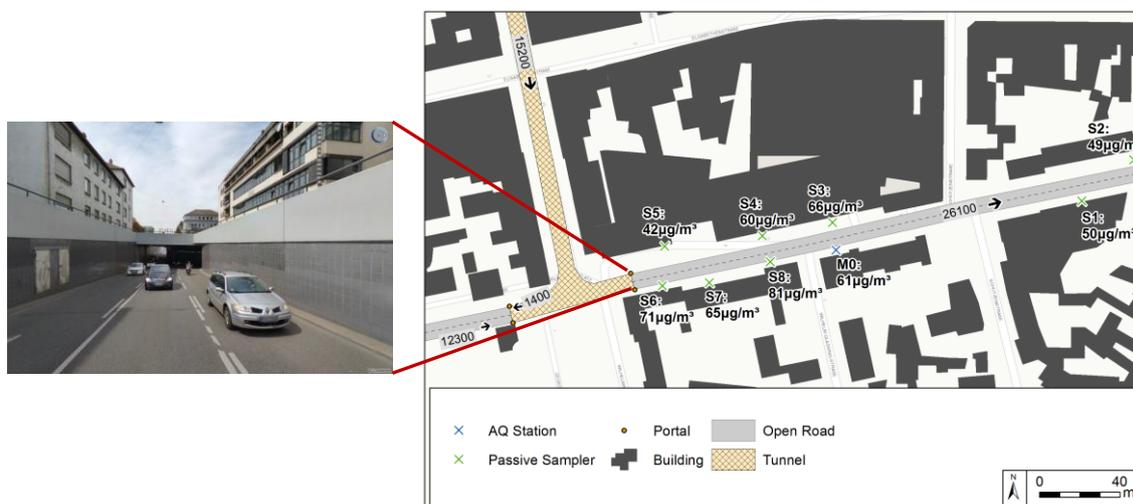
**Figure 1.** Tunnel exit portal and studied road transect with 26 100 ADTV and monitored AM NO<sub>2</sub> concentrations.
