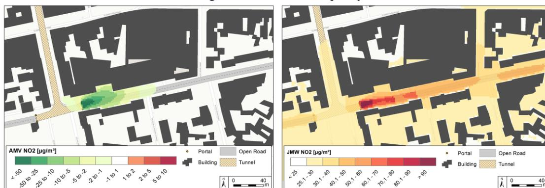
**Figure 5.** Difference AM NO<sub>2</sub> portal air management mitigation scenario – base (left). AM NO<sub>2</sub> for 50 % traffic reduction scenario (right).
