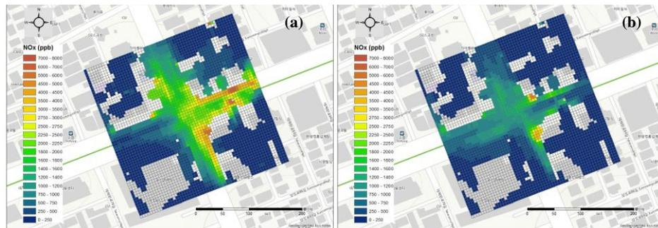
**Figure 5.**  $\text{NO}_x$  concentration results from CFD simulation using traffic emissions with  $5\text{m} \times 5\text{m}$  grid resolution for (a) peak and (b) off-peak scenario.
