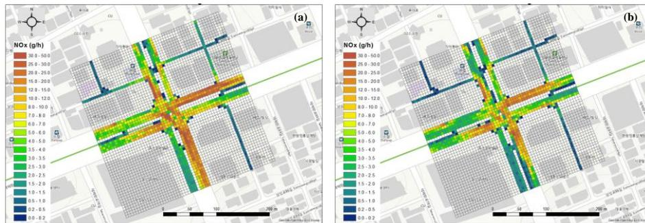
**Figure 4.**  $\text{NO}_x$  emission results with  $5\text{m} \times 5\text{m}$  grid resolution for (a) peak and (b) off-peak hour.
