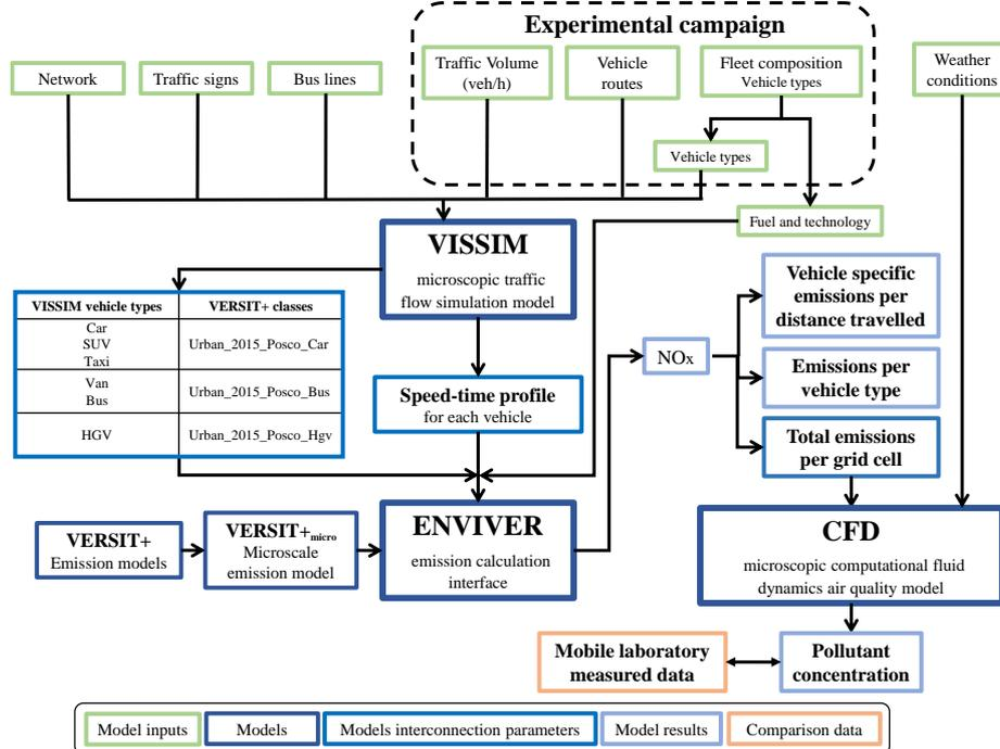
**Figure 2.** General flowchart of the modelling system including inputs and outputs for comparison with mobile laboratory measured data.
