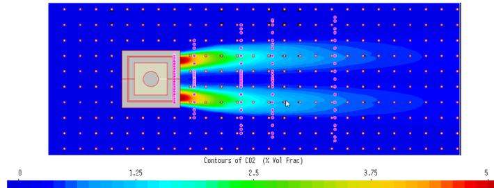
**Figure 2.** Site features and concentration contours (% Vol Frac) on ground level for Case B
