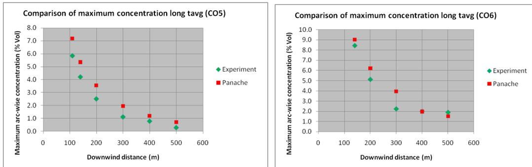
**Figure 1.** Comparison between experimental and numerical (modelled) maximum arc-wise concentration longest time average for CO5 and CO6
