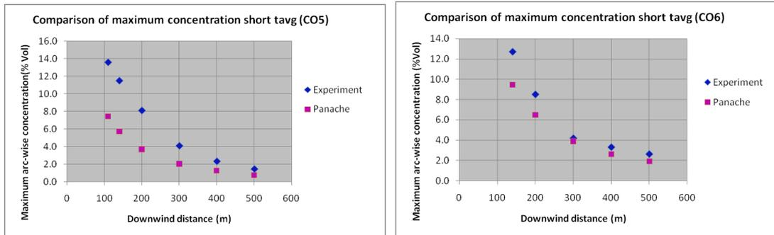
**Figure 1.** Comparison between experimental and numerical maximum arc-wise concentration short time average for CO5 and CO6
