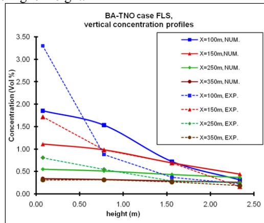
Figure 7. Comparison of measured and simulated concentrations for vertical profiles for FLS case
