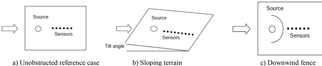
**Figure 4.** BA-Hamburg setup for: a) Unobstructed terrain (DA0120), b) Sloping terrain (DAT637) and c) Downwind fence (DA0532)
