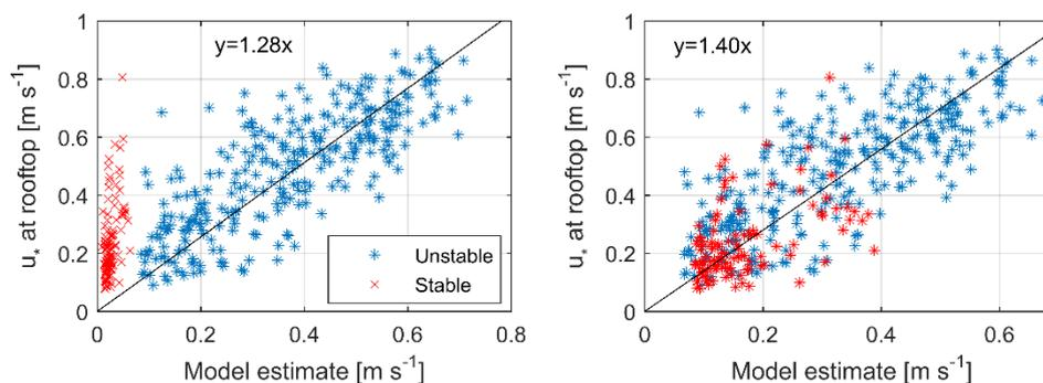
**Figure 3.** Model estimates of rooftop friction velocity compared with observations. Left panel: Accounts for stability. Right panel: Assumes neutral conditions in urban area.
