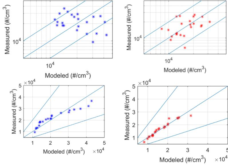
**Figure 2.** Scatter and quantile-quantile plot of measured and modeled values. Left panel: wall barrier. Right panel: wall-vegetation barrier.
