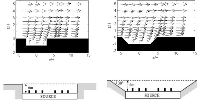
**Figure 1.** Two configurations studied in the wind tunnel. Left panels shows the flow field and source configuration for the 6 m depressed road. The right panels show the effects of angled side walls.
