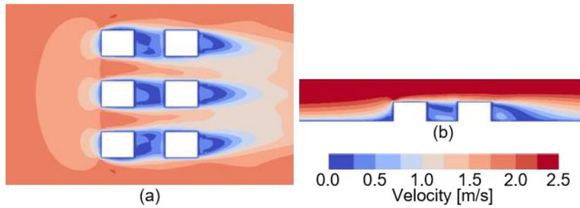
**Figure 3.** Velocity field at (a) 3.25 m high, (b) center of the north-south direction.
