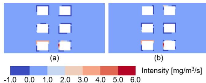
**Figure 6.** Estimated Source location and intensity when “correct” sources are (a) located at A in figure 2(a), (b) located at A and B in figure 2(a).
