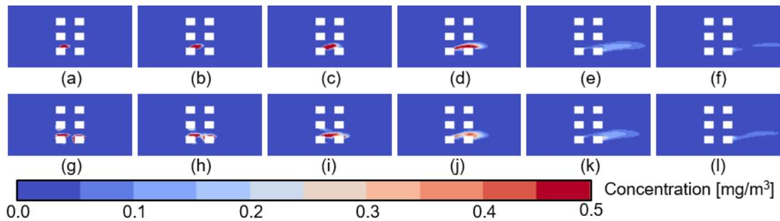
**Figure 4.** The concentration fields (a-f) calculated with “correct” source, and (g-l) estimated by VCA method, when the “correct” source is located A (figure 2(a), at  $t = 4, 8, 16, 32, 64, 96$  s.
