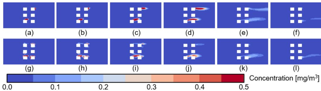
**Figure 5.** The concentration fields (a-f) calculated with “correct” sources, and (g-l) estimated by VCA method, when the “correct” sources are located A and B (figure 2(a)), at  $t = 4, 8, 16, 32, 64, 96$  s.
