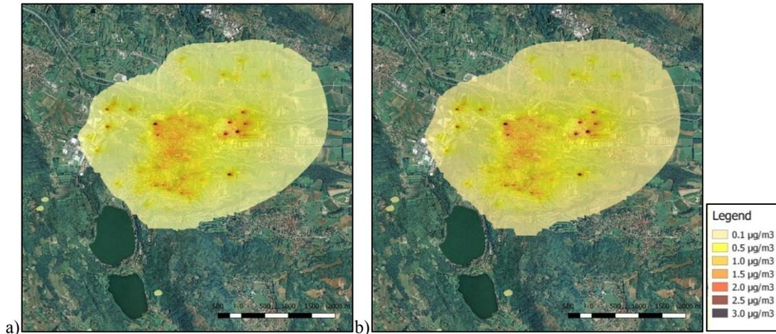
**Figure 4.** Concentration of PM from the emissions of biomass boilers with increased (a) and decreased (b) of 2°C temperature input data
