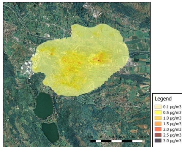
**Figure 5.** Concentration of PM from the emissions of biomass boilers in the hypothesis of improved buildings energy performance
