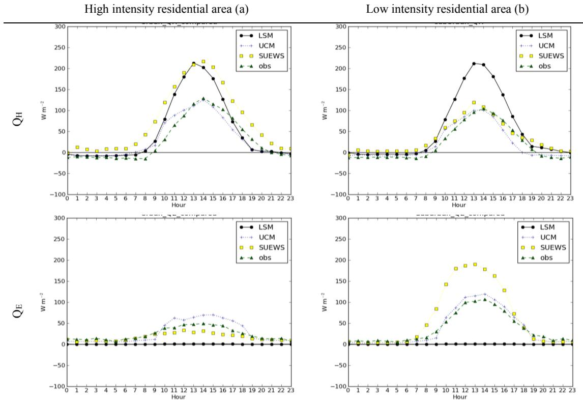
**Figure 2.** Modelled and measured five-months averaged energy balance at the high and low intensity residential areas.  $Q_E$ : latent heat flux and  $Q_H$ : sensible heat flux.
