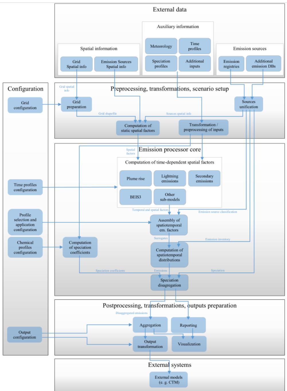
**Figure 1** Structure of the new emission processor. The scheme shows basic layers of the processor, flow of the data and modules dependency (from Juruš et al., 2016).
