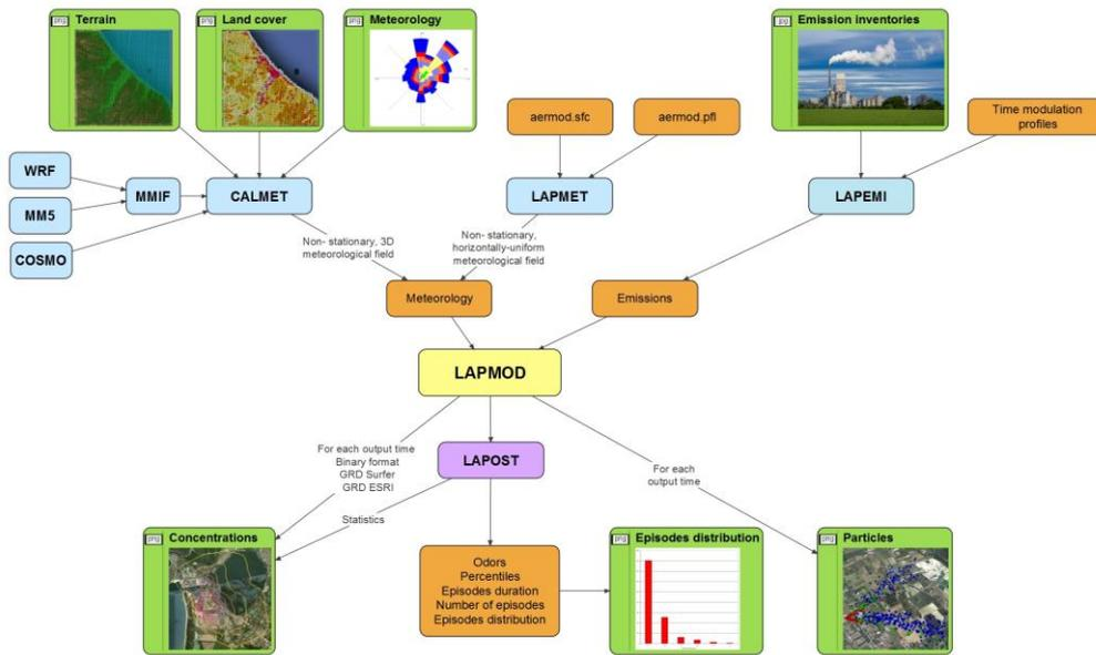
Figure 1. Structure of the LAPMOD model system.
