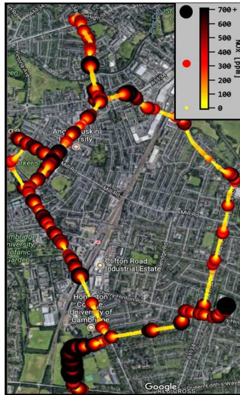
**Figure 1.** An overview map showing NO<sub>x</sub> concentrations from a Diesel vehicle driven around Cambridge. Concentrations higher than 700 ppm per GPS point are circles coloured in black, at the largest diameter.
