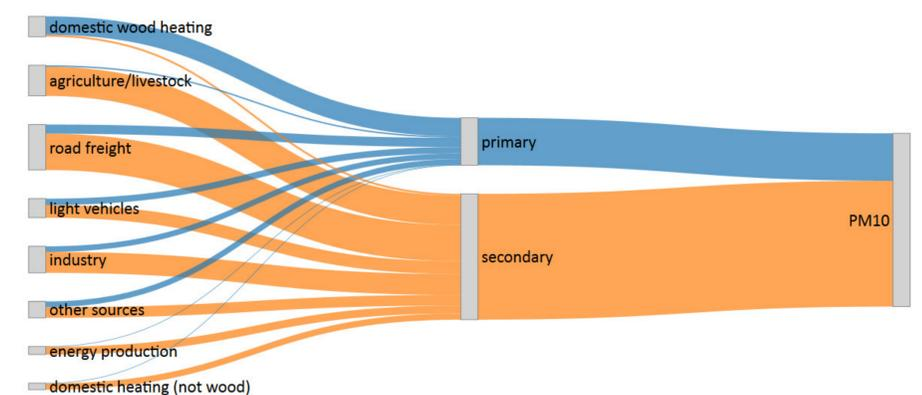
Figure 2: The AF allows expressing anthropogenic PM10 precursors in terms of "PM10 equivalent" in the domain. In this Sankey diagram (Sankey, 1896) the width of the connections is proportional to the "flow" of PM10 equivalent mass in the Emilia-Romagna region. On the left side, emissions are aggregated by emission sector; in the center, aggregated by category.
