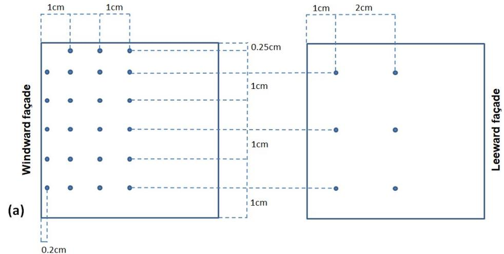
Extra pressure taps near the edges of the wall →
