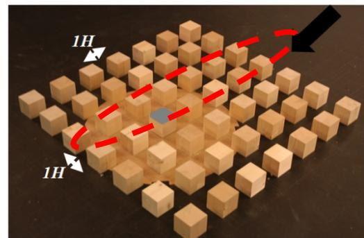
Drag force and pressure measurements were performed separately on individual (target) cubes
