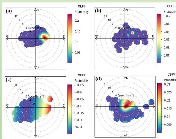
The NO<sub>x</sub> pollutant roses for the four simulation periods performed using SWIFT wind data for the source point at the plant stack elevation and the hourly NO<sub>x</sub> ground simulated concentrations in a 100 m x 700 m area over the Eastern slope of Mount Titano were used to obtain conditional bivariate probability functions (CBPF) (figure at left).
