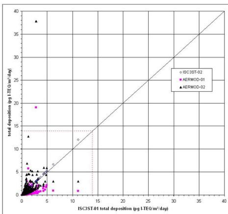
Figure 2: scatterplots of total deposition results obtained with AERMOD and ISC3ST simulations. The dashed line indicates the reference value adopted (14 pg I-TEQ/m<sup>2</sup>/day).
