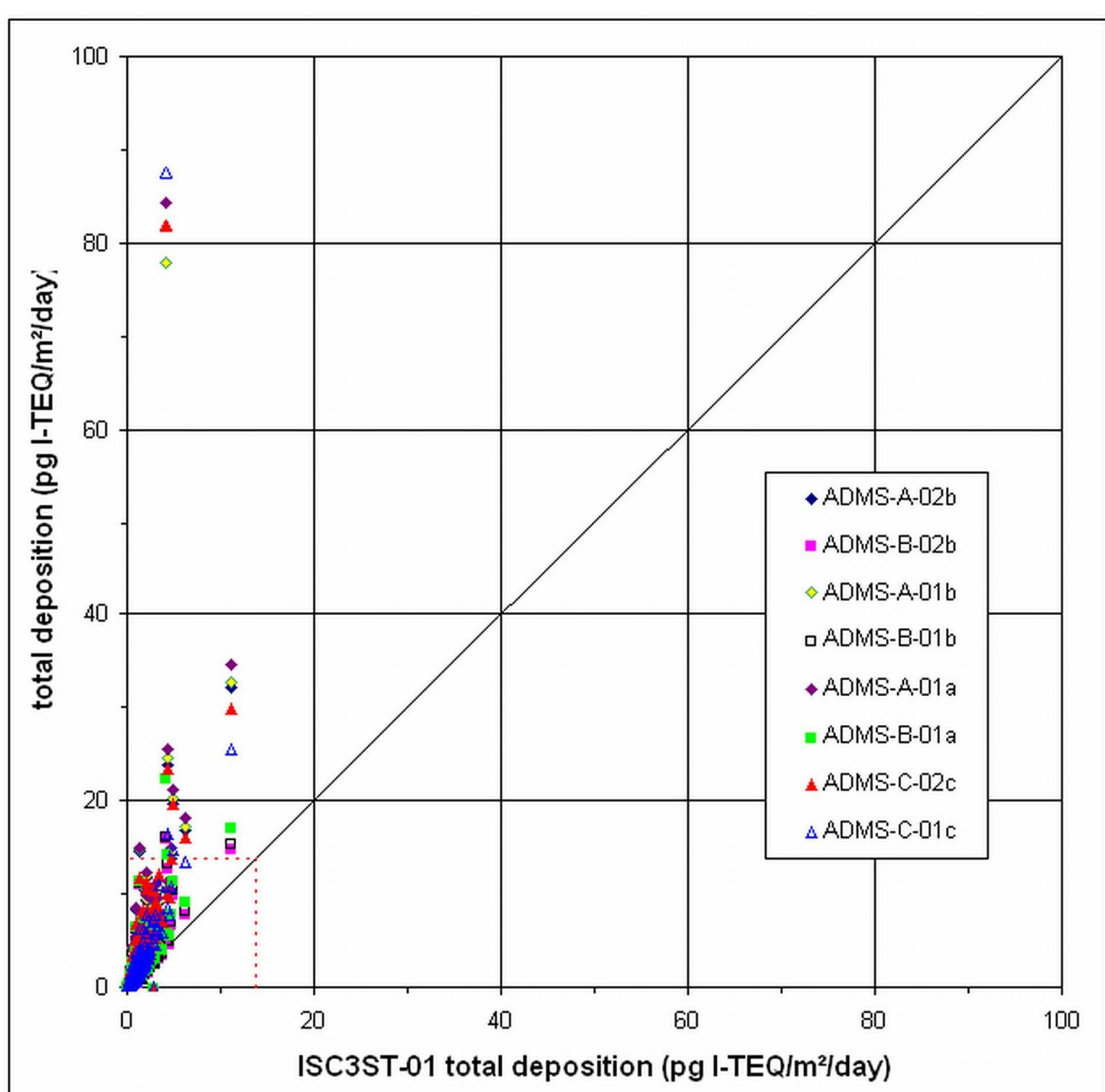
Figure 3: scatterplots of total deposition results obtained with ADMS simulations respect those of ISC3ST-01. The dashed line indicates the reference value adopted (14 pg I-TEQ/m<sup>2</sup>/day).
