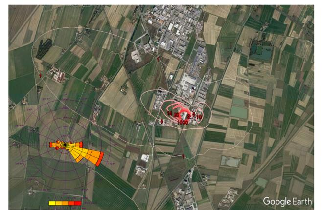
Figure 5: qualitative representation with isolines of the on-soil total deposition estimates (pg I-TEQ/m<sup>2</sup>/day) obtained by the ADMS-A-01a simulation. In the left corner it is shown the surface winds rose.
