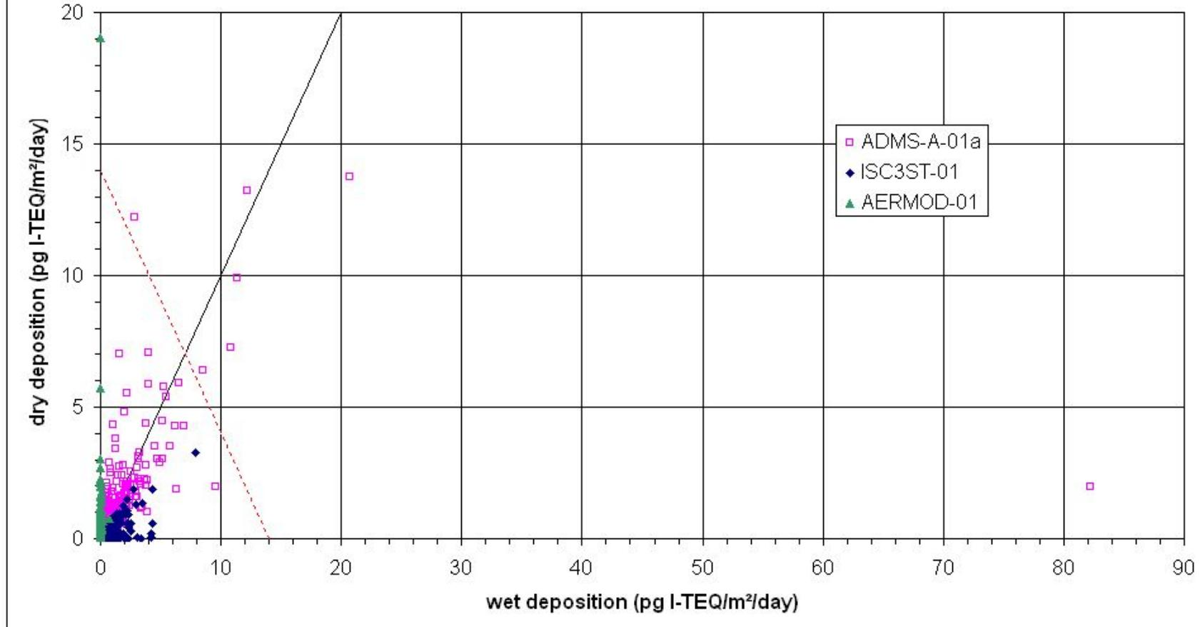
Figure 4: comparison between dry deposition and wet deposition values obtained in the simulation ISC3ST-01, AERMOD-01 and ADMS-A-01a. The dashed line indicates the reference value adopted (14 pg I-TEQ/m<sup>2</sup>/day).
