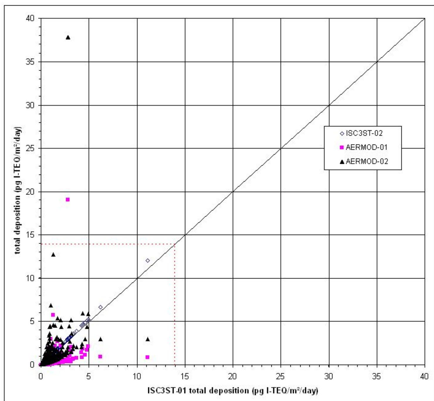
Figure 2: scatterplots of total deposition results obtained with AERMOD and ISC3ST simulations. The dashed line indicates the reference value adopted (14 pg I-TEQ/m<sup>2</sup>/day).
