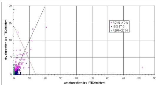
Figure 4: comparison between dry deposition and wet deposition values obtained in the simulation ISC3ST-01, AERMOD-01 and ADMS-A-01a. The dashed line indicates the reference value adopted (14 pg I-TEQ/m<sup>2</sup>/day).
