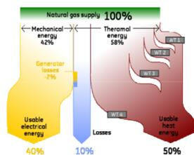
**Principle:** CCHP is a natural gas-fired, it produces 40% of usable electricity and 50% heat energy to be used for hot/cold water and heating
