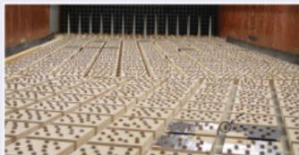
Figure: Example of idealized neighborhood in wind tunnel from (Garbero et al.,2010)
