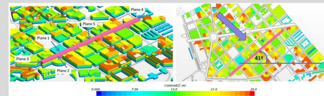
Fig. 5. Planes used for street ventilation assessment (left) and street orientation and wind direction (right).
