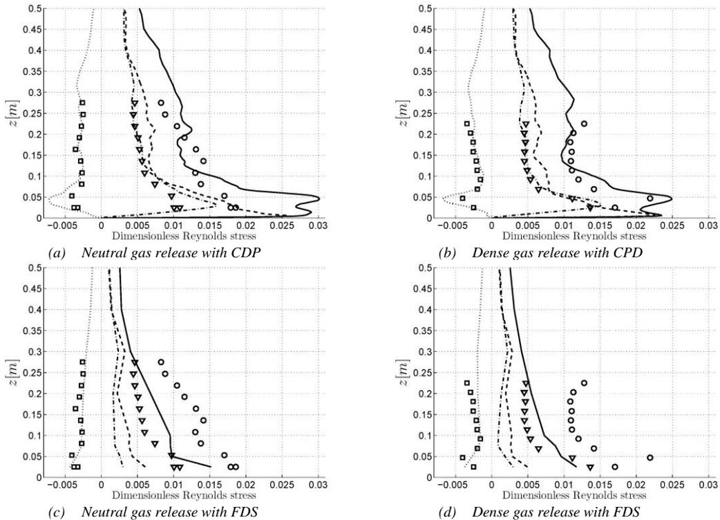
**Figure 3.** Vertical variation of Reynolds stresses at  $(x,y)=(9.5h,0)$ . Symbols illustrate experimental measures and lines show numerical result.  $\langle u'u' \rangle$  ( $\circ$ , —),  $\langle v'v' \rangle$  (---),  $\langle w'w' \rangle$  ( $\nabla$ , -.-) and  $\langle u'w' \rangle$  ( $\square$ , .....).
