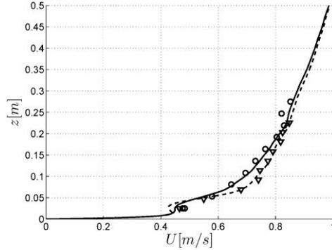
**Figure 2.** Vertical profiles of mean streamwise velocity for neutral and dense gas release at  $(x,y)=(9.5h,0)$ . Symbols denote experimental measures (neutral  $\circ$ , dense  $\nabla$ ) and lines numerical results (neutral —, dense ---) using the CDP solver.
