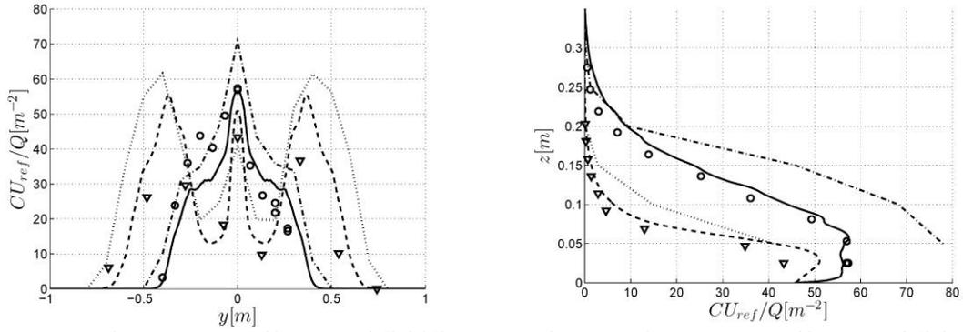
(a) Lateral concentration profile at  $(x,z)=(9.5h,0.25h)$  (b) Vertical concentration profile at  $(x,y)=(9.5h,0)$
