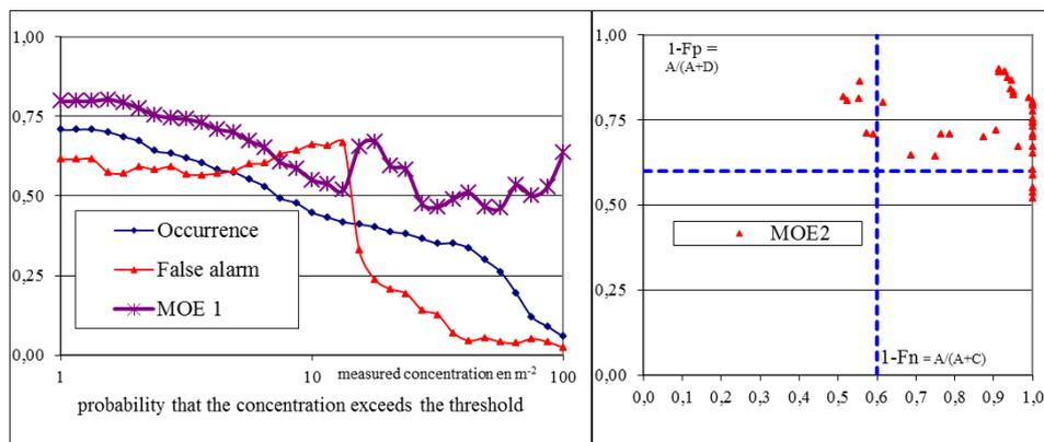
**Figure 4.** Left panel, false alarm represent ~60% for low concentrations  $< 10\text{m}^{-2}$  in streets a few hundred meters from the source. Much better False Alarm rates ( $< 25\%$ ) are obtained if we cut at  $10\text{m}^{-2}$ . MOE1  $> 50\%$  is acceptable for validation purpose. Right panel, points are in general centered in a 60% square. A few false positives and false negatives in far field are probably due to an orientation shift between experiment and simulation.
