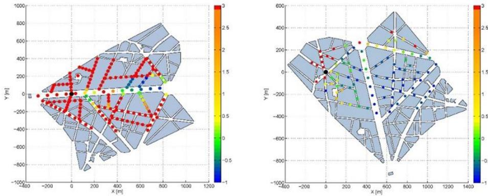
**Figure 3.** Comparison of ARGOS concentrations with wind tunnel measurements (Source position S1 to the left and S3 to the right). Positive values indicate factors of over-prediction and negative values indicate factors of under-prediction. The black dot shows the position of the source. The wind direction is from left to right in the figures.
