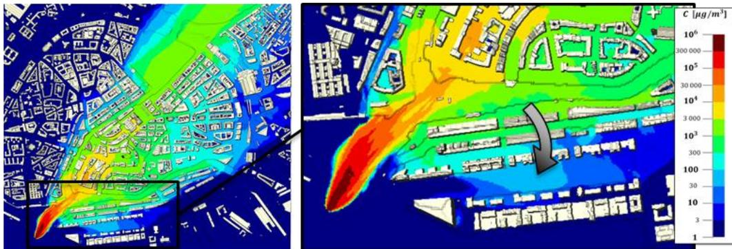
Figure 5. Direction of the plume propagation opposite to the main flow direction.
