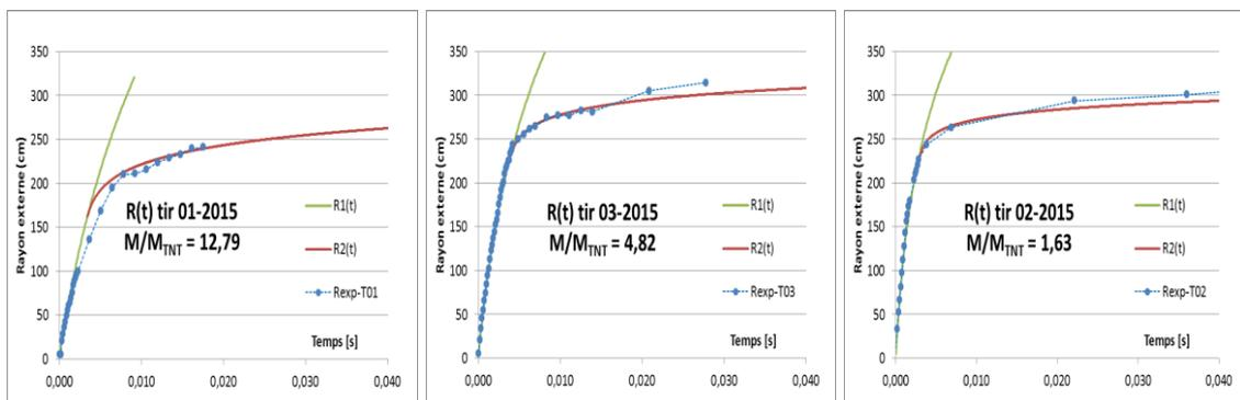
**Figure 2.** D2R2 results compared to CEA experiments (time evolution of the external radius).
