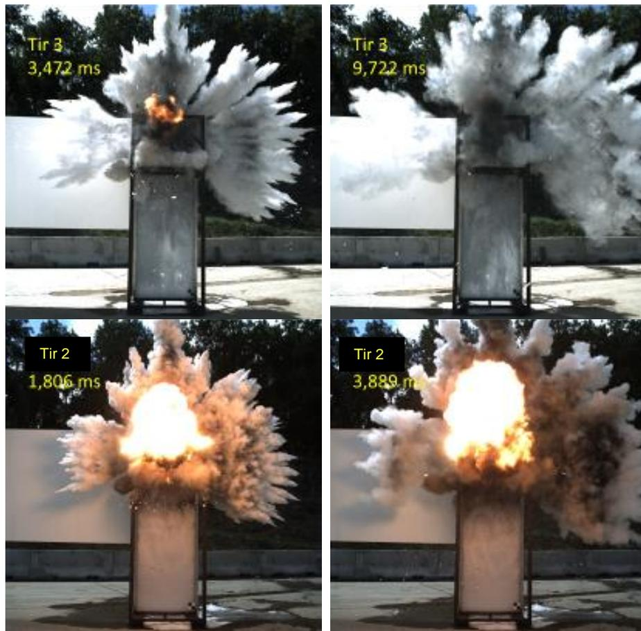
**Figure 1.** Change of morphology for two mass ratios (from top to bottom: 4.8 and 1.6).
