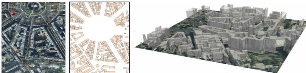
**Figure 4.** From left to right: Google Maps® view, BD TOPO shapefile, and HI2LO geometry after processing.
