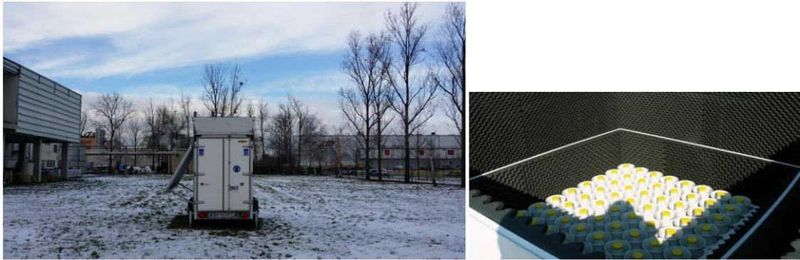
**Figure 2.** Location of the METEK SODAR east of the Energy Base building (left) and SODAR antenna array (right)
