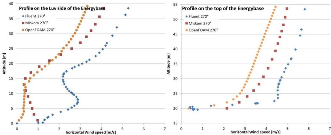
**Figure 6.** Profiles of the horizontal wind speed on the luv side (left) and at the SWT site on top of the Energy Base building (right) simulated with FLUENT, MISKAM and OpenFOAM for the 270 ° flow case.
