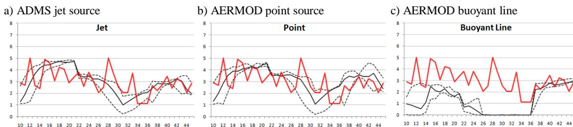
**Figure 5.** Short-term odour results for Whitelees a) ADMS jet, b) AERMOD point and c) AERMOD buoyant line sources; observations shown in red, minimum, median and maximum modelled values shown in black, where range of modelled values corresponds to wind direction adjustments of  $\pm 15^\circ$ . Horizontal axis shows transect receptor number, as shown in Figure 1b).
