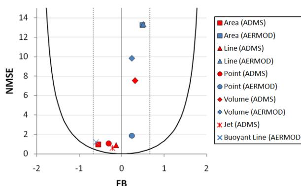
**Figure 3.** NMSE against fractional bias (FB) for all source types; buildings explicitly modelled with point sources only. Black line indicates minimum NMSE possible for FB.
