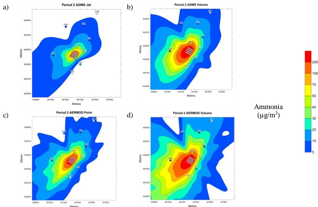
**Figure 4.** Period average  $\text{NH}_3$  for Whitelees 'Run 2': a) ADMS jet, b) ADMS volume, c) AERMOD point and d) AERMOD volume. Observations shown by the circles, the buildings are shown in grey (modelled in c)).
