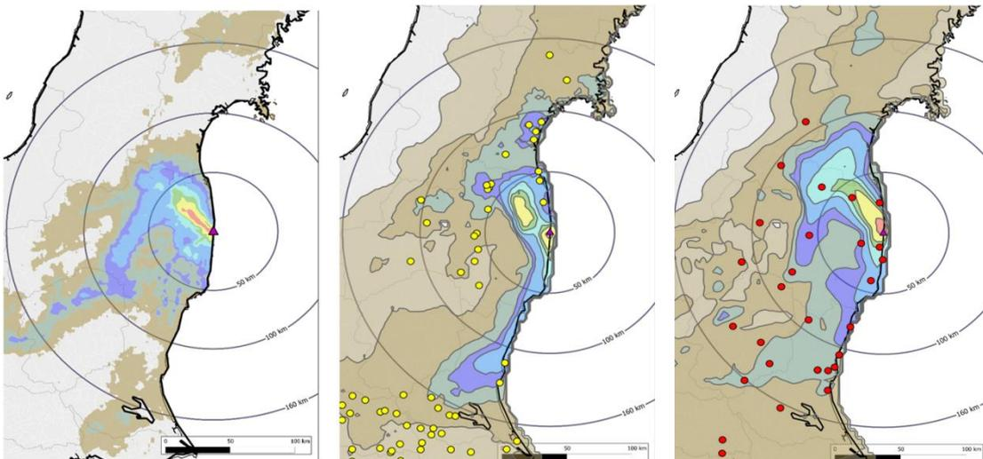
**Figure 4:** Map of cumulated Cs-137 surface deposition observed on April 1, 2011 (left). Comparison of the cumulative  $^{137}\text{Cs}$  ground deposition from simulations forced with inverted ST-1: (middle) and ST-2 (right). Circles represent the location of the stations used in the inversion. Red circles are dose rate observations and yellow circles are Tsuruta  $^{137}\text{Cs}$  air concentrations observations. Values are given in  $\text{Bq/m}^2$ .
