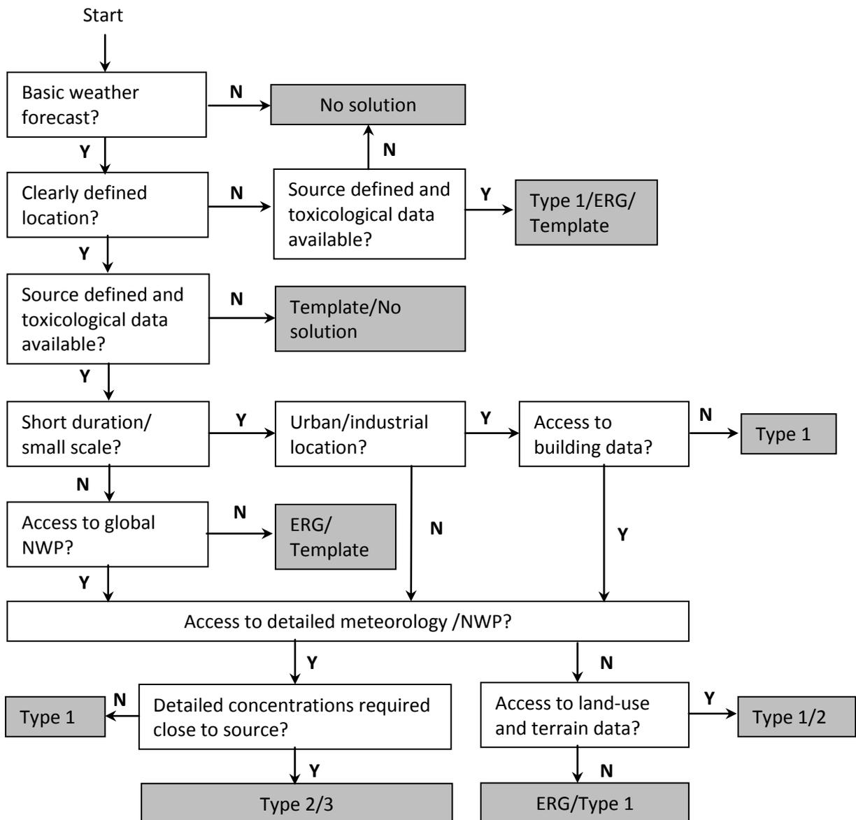
**Figure 1.** Emergency response modelling selection flowchart.
