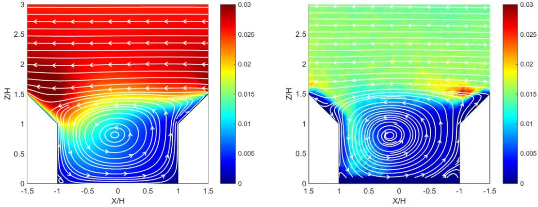
**Figure 5.** Non-dimensional mean Turbulent Kinetic Energy ( $TKE/U^2$ ) fields(color map) with streamlines (white lines) from numerical (left side) and laboratory (right side) simulations, for pitched roof and  $W/H = 2$ .
