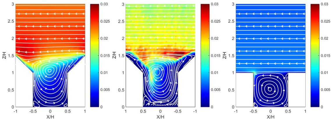
**Figure 4.** Non-dimensional mean Turbulent Kinetic Energy ( $TKE/U^2$ ) fields (color map) with streamlines (white lines) for  $W/H = 1$ : numerical (left side) and laboratory (center) simulations, for pitched roof, numerical simulations for flat roof (right side).
