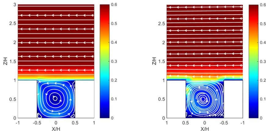
**Figure 1.** Non-dimensional mean velocity  $u/U$  fields (color map) with streamlines (white lines) from numerical (left side) and laboratory (right side) simulations, for flat roof and  $W/H = 1$ .
