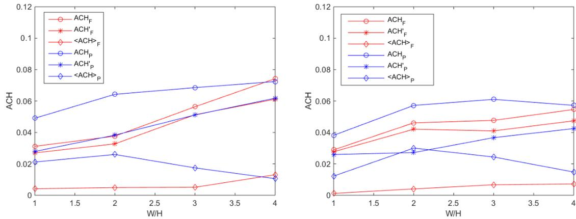
**Figure 6.** ACH versus  $W/H$  from numerical (left side) and laboratory (right side) simulations; flat roof values are plotted with red lines, pitched roof values with blue lines; total ACH is plotted with circles, mean ACH component with asterisks and turbulent ACH component with rhombi.
