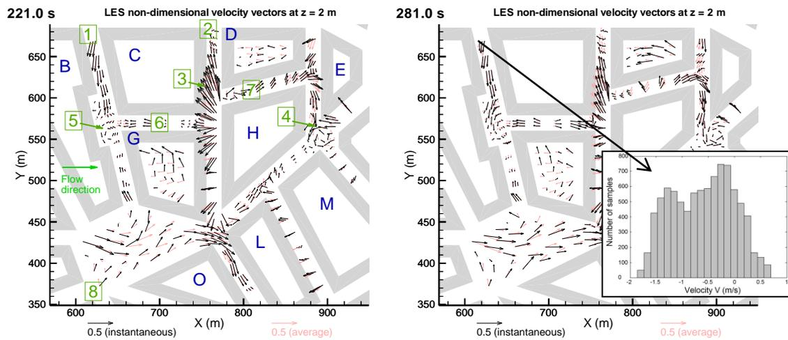
**Figure 3.** Two frames of a 9000 s video showing the LES instantaneous velocity vectors at  $z = 2 \text{ m}$ . In the inset the probability density function of the  $V$  velocity at point 1 is plotted, which shows bimodal behaviour
