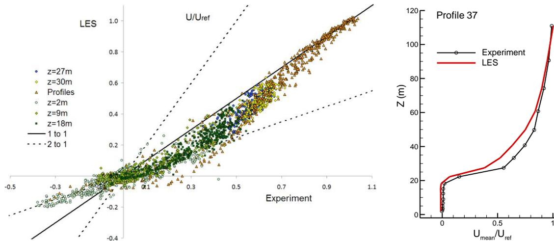
**Figure 2.** Left: Comparison of experimental and LES values of mean velocity  $U_{mean}$  at all measurement points. Right: Vertical velocity profiles of experiment and LES at point 37, between buildings **B** and **G** (Figure 1)
