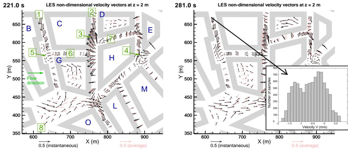
**Figure 3.** Two frames of a 9000 s video showing the LES instantaneous velocity vectors at z = 2 m. In the inset the probability density function of the V velocity at point 1 is plotted, which shows bimodal behaviour
