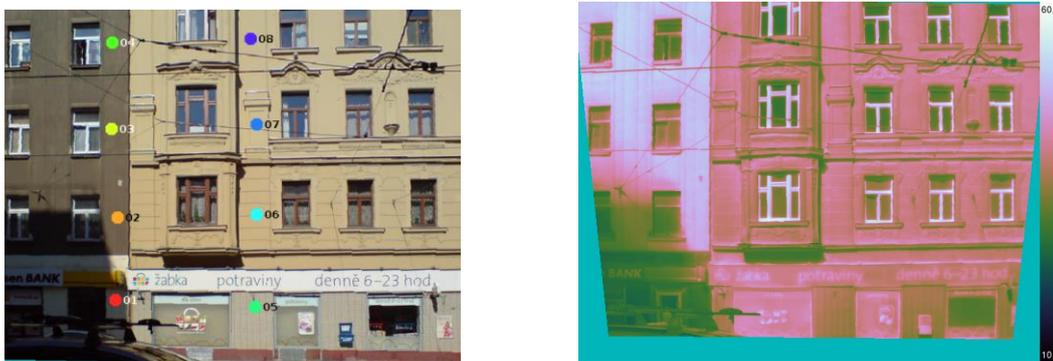
**Figure 2.** Onsite measurement campaign. Left: east facing wall in visible spectrum with reference points. Right: east facing wall in infrared spectrum (8:11 CET).
