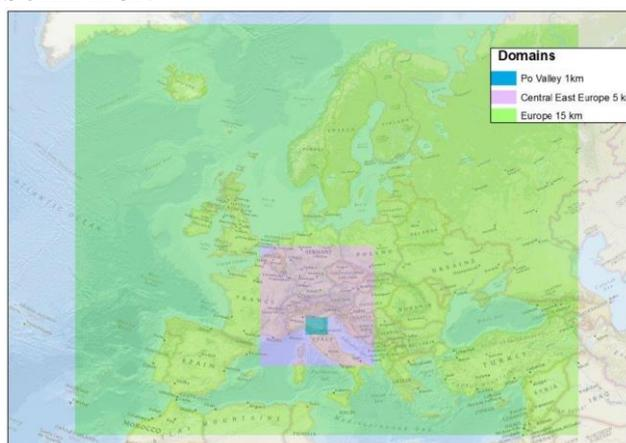
**Figure 1.** The sequence of nests in EURAD-IM. The coarse grid is Europe with 15×15 km<sup>2</sup> resolution which includes two nest domains: the central Europe and the area of Po Valley in Italy with 5×5 km<sup>2</sup> and 1×1 km<sup>2</sup> resolution, respectively.
