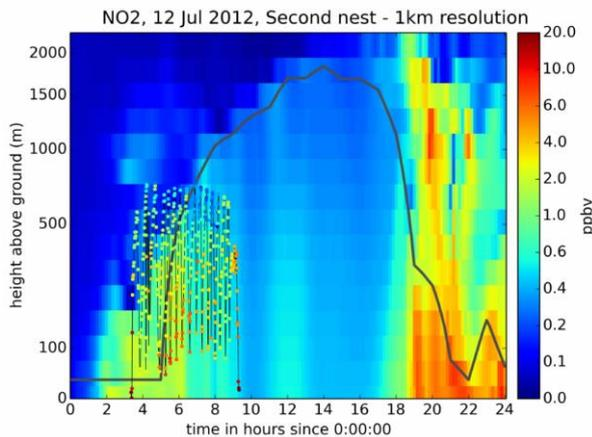
**Figure 4.** Hovmöller plot. Timeseries of PBL and the vertical NO<sub>2</sub> concentrations at SPC: observations from the flight campaign (dots) and model results from concerning the Po valley domain (background).
