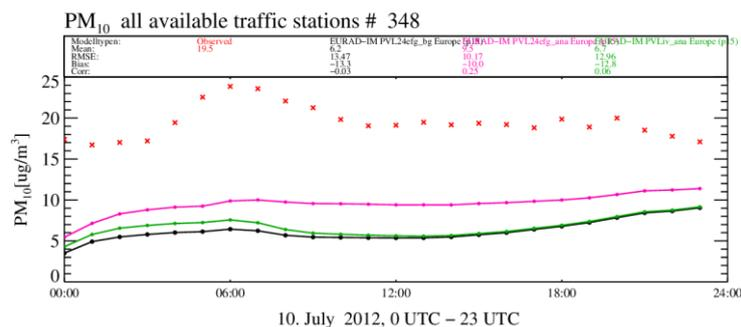
**Figure 5.** Timeseries for PM<sub>10</sub> concerning the average of all AirBase station with traffic influence over the European domain. Observations are given in red, background in black; analyses with 6h of assimilation window in green and with joint optimization of aerosol and gas-phase are in pink.
