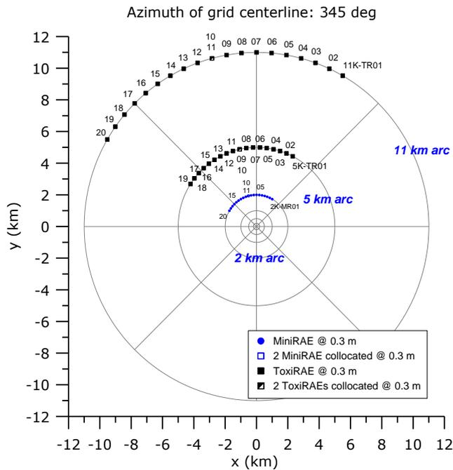
**Figure 3.** JR II 2015 sampler grid for 2, 5, and 11 km arcs.
