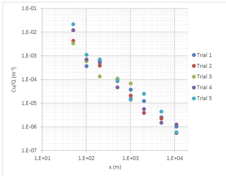
**Figure 4.** Observed JR II 2015 arc max 1 sec avg Cu/Q ( $\text{m}^{-2}$ ) vs x (m).
