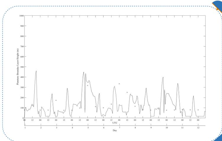
**Figure 4.** Evolution of the planetary boundary layer height along June 2009: (-) WRF, (o) ceilometer.
