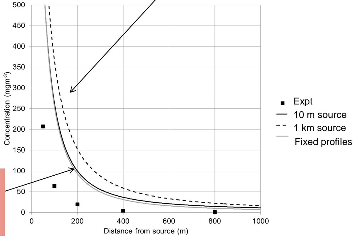
Release near the inlet is similar to case with fixed profiles
