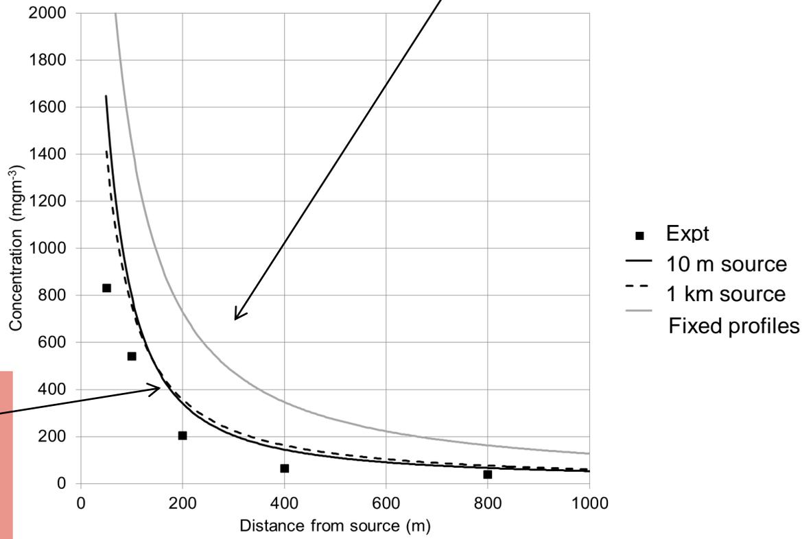
Release near the inlet is similar to release at 1 km downwind
