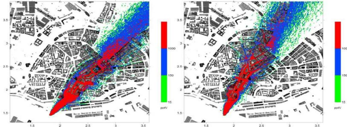
Field experiment / continuous release - Cross-section near the ground (PMSS diagnostic)
