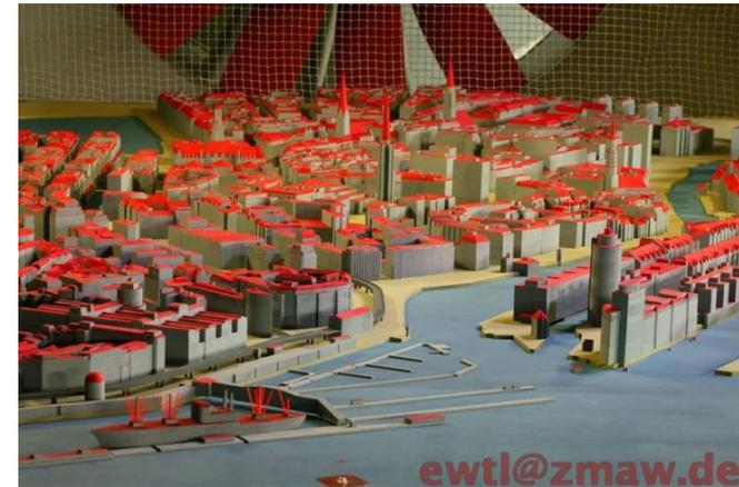
City centre of Hamburg (left) and its mock-up in the WOTAN wind tunnel (right)
