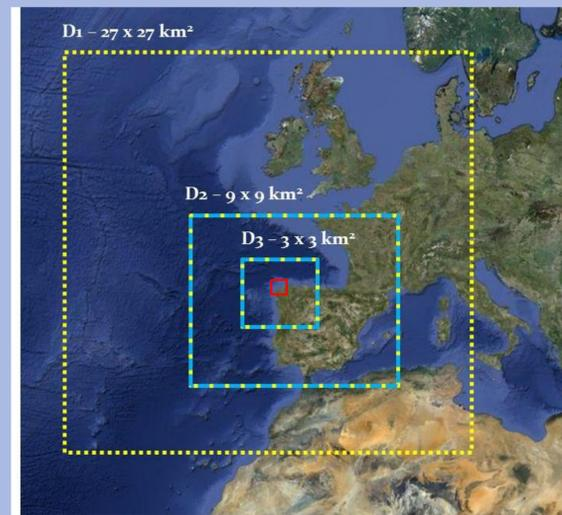
Figure 2. Nested WRF simulation domains (resolution: D1: 27x27 km<sup>2</sup>; D2: 9x9 km<sup>2</sup>; D3: 3x3 km<sup>2</sup>), to provide meteorological inputs to CALMET model domain (□; 0.5x0.5 km<sup>2</sup> resolution).
