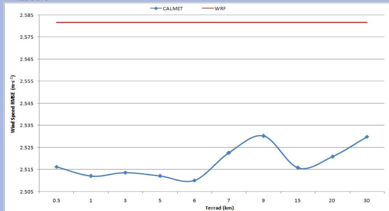
Figure 3. Wind speed RMSE variation from WRF simulation (3x3 km<sup>2</sup> resolution) and CALMET simulations with different TERRAD values.
