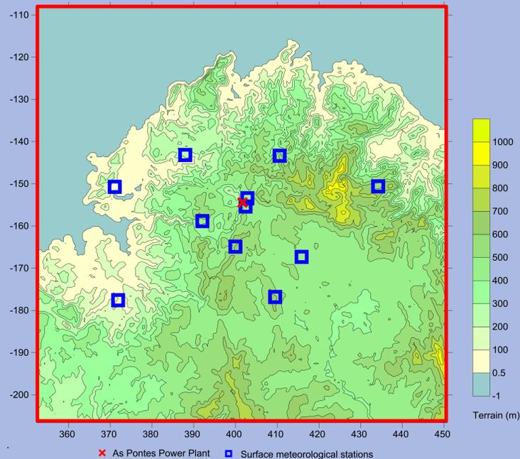
Figure 1. Location (UTM coordinates) and digital elevation model (asl-m) of the CALMET simulation domain inside the D3 domain, with the location of meteorological surface sites for model assessment. Terrain values [-1,0.5] correspond to sea level.
