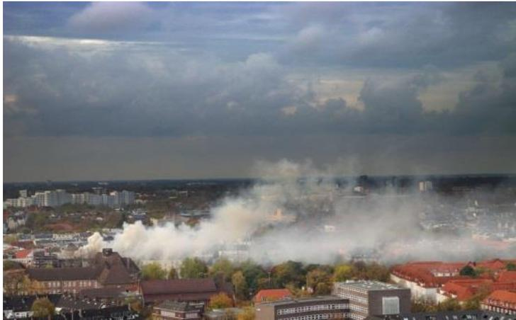
Continuous 45-minutes release of SF6 with a flow rate of 2 g/s, from a building in the harbor area.
