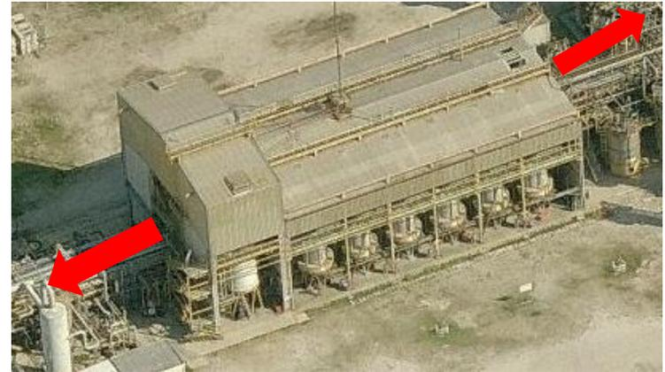
Vinyl Chloride Monomer accidentally released inside a building in a liquid state and evaporated causing high concentrations in the air outside the building.
