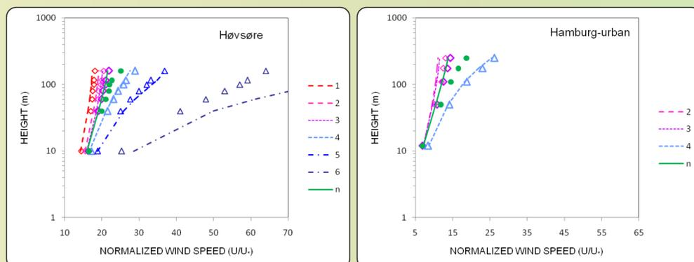
Figure 1. Comparison of normalized wind profiles (lines) with measurements (symbols) as a function of stability for Høvsøre (left panel) and Hamburg (right panel)
