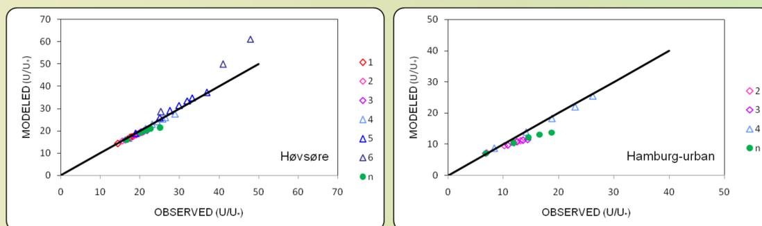
Figure 2. Comparison of modeled normalized wind profiles with measurements as a function of stability (symbols) for Høvsøre (left panel) and Hamburg (right panel). The line indicates the best fit.
