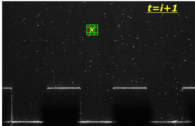
**FTV (Feature Tracking Velocimetry)** compares windows only where the motion detection may be successful: tracking of regions with high luminosity gradients (i.e. features).
