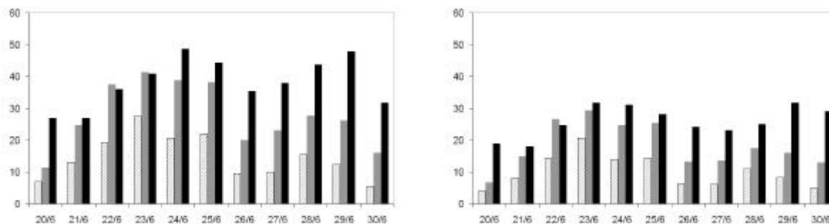
Fig. 3; summer  $PM_{10}$  daily mean concentration levels ( $\mu g/m^3$ ) at Borgaro (left) and Druento (right) stations; black bars refer to measured values, light grey bars refer to base case and dark grey bars to Test 2.
