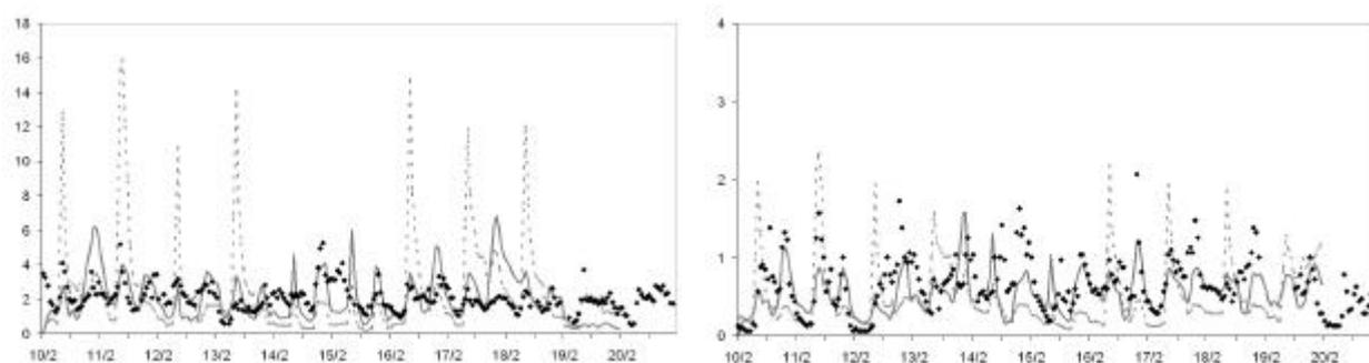
Fig. 4; winter benzene hourly concentration levels (ppb) at Torino-Consolata (left) and Cuneo (right) stations; dots refer to measured values, dotted light grey line to base case and solid dark grey line to Test 3.
