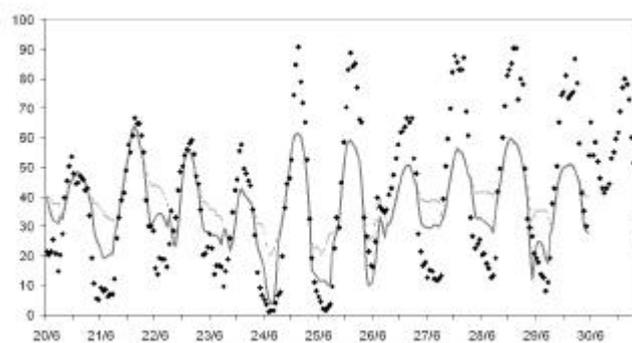
Fig. 2; Summer ozone hourly concentration levels (ppb) at Druento station; dots refer to measured values, dotted light grey line to base case and solid dark grey line to Test 1.
