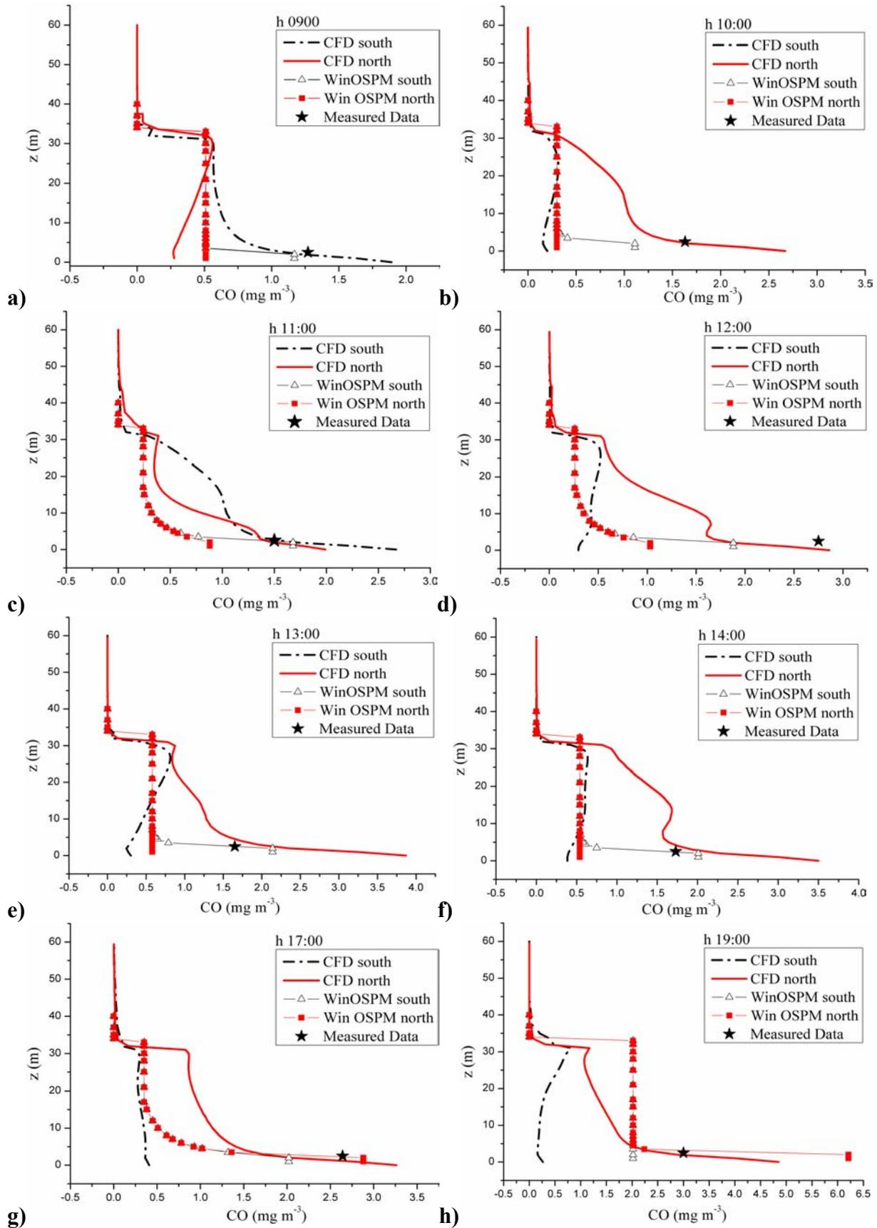
Figure 4. Vertical CO concentration profiles computed with WinOSPM and CFD on the North and South sides of the canyon.
