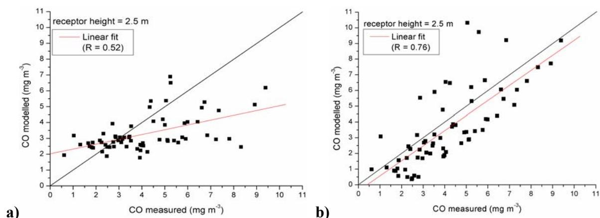
Figure 3. Measured vs. modelled CO concentration at receptor location ( $z = 2.5$  m) by using a) an unmodified version of WinOSPM, and b) a reduction factor for the wind speed 10 times higher than the default value set in WinOSPM. Linear fit and correlation coefficients ( $R$ ) are reported for both cases.
