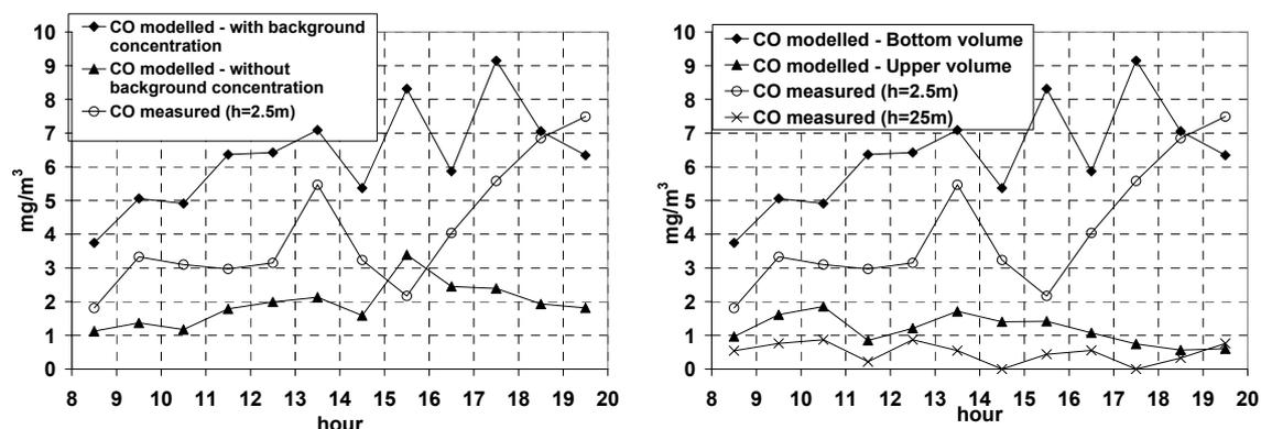
Figure 2 Comparison between CFD simulations and monitoring data
