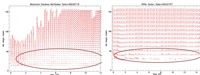
Fig. 4. ANL BG (left, July 19, 2003) and PNNL (right, July 27, 2003) (mini-) SODARs wind vector profiles as a function of time (at night) and altitude.
