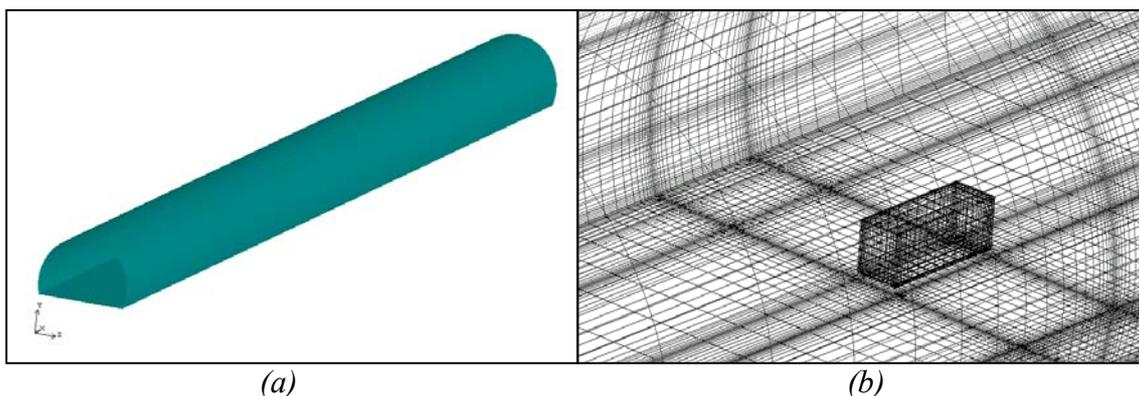
Fig. 1; Tunnel geometry and mesh refinement close to a car in the middle lane approximated as a simplified block
