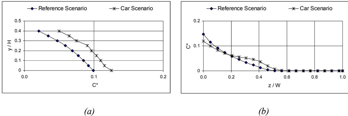
Fig. 4; Non-dimensional concentration profiles at 80 m from the tunnel's exit in the case of the moving buses, for the two scenarios in the (a) vertical and (b) lateral directions.
