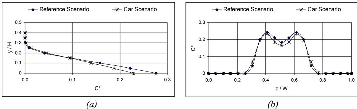
Fig. 2; Non-dimensional concentration profiles at 80 m from the tunnel's exit in the case of the moving cars for the two scenarios in the (a) vertical and (b) lateral directions.
