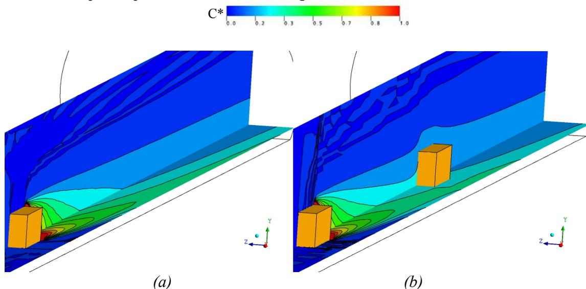
Fig. 5; Non-dimensional concentration fields in the case of the moving buses, for the two scenarios in vertical and horizontal planes.
