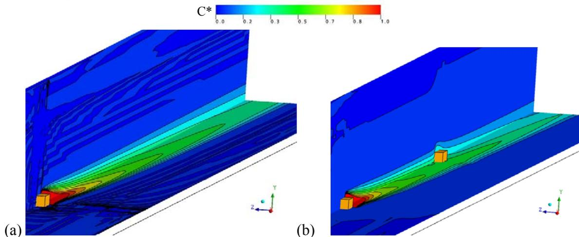
Fig. 3; Non-dimensional concentration fields in the case of the moving cars for the two scenarios, in vertical and horizontal planes.
