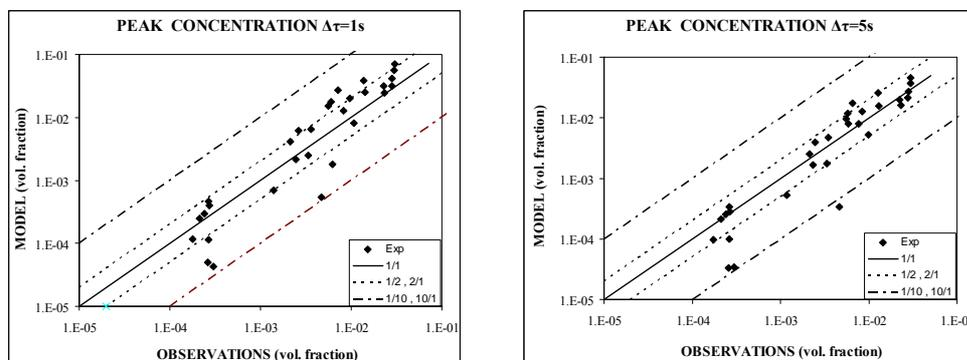
Fig 3; Estimated peak concentrations at (a) 1 s and (b) 5 s
