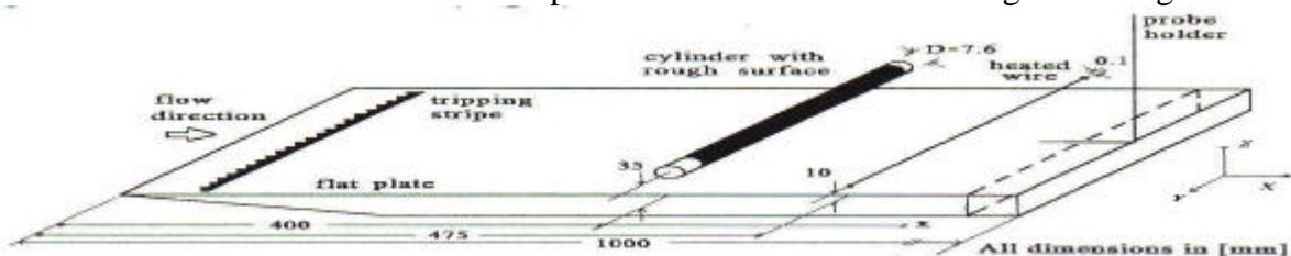
Fig 1; The experimental setup.
