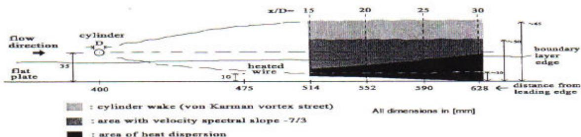
Fig. 2; Schematic representation of the experimental flow created in the wind tunnel.
