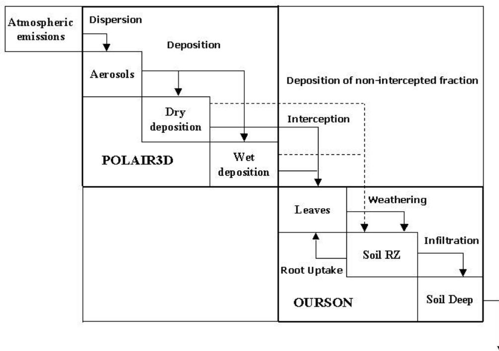
Fig. 1; Features, Events and Processes taken into account in the POLAIR3D and OURSON models.
